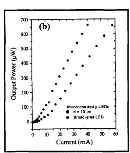
We have succeeded in interconnecting hundreds of III-nitride micro-size LEDs (of the order of 10  $\mu$ m in diameter) – see Figure 2 – so that they are turned on and off simultaneously and fit into the same device area as a conventional LED of about 300 x 300  $\mu$ m<sup>2</sup>.
